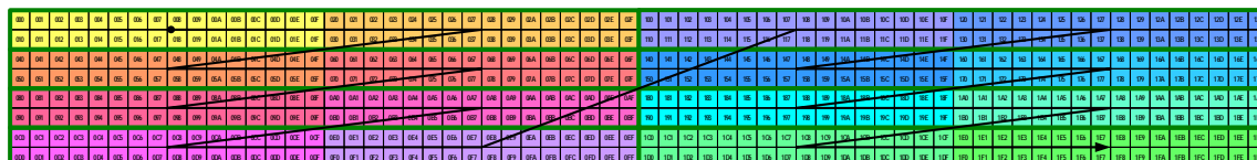
Figure 45: Block Linear (GPU 16Bx2 kind with Tegra X1 Sector Ordering)
